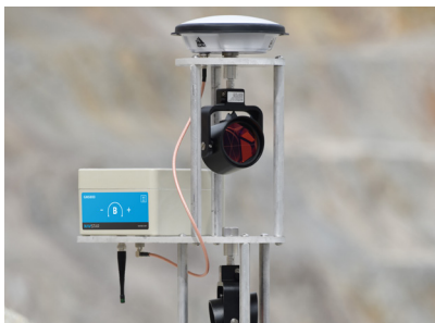
GMS800s can be used with NavStar's ACAL Advanced Calibration system for high precision prism monitoring.
